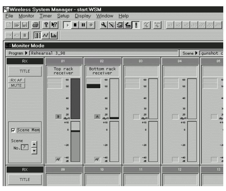
All screen functions are the same as in the Monitor screen, except that there is a single RF Level meter for each receiver. This meter shows the RF signal strength being received by the antenna currently in use, and the legend beside it shows whether the "A" or "B" antenna is the current one. In addition, there are fewer items in the Status Display; only Audio Frequency (Rx AF) on/off and Mute on/off are shown (as in the Monitor screen, when Mute is on, the box is colored red).
